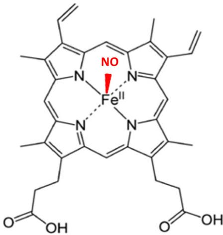
**Fig. 4.** A nitrosyl-heme compound containing the NO group directly bound to a metal (Fe) giving a metal-NO moiety.
